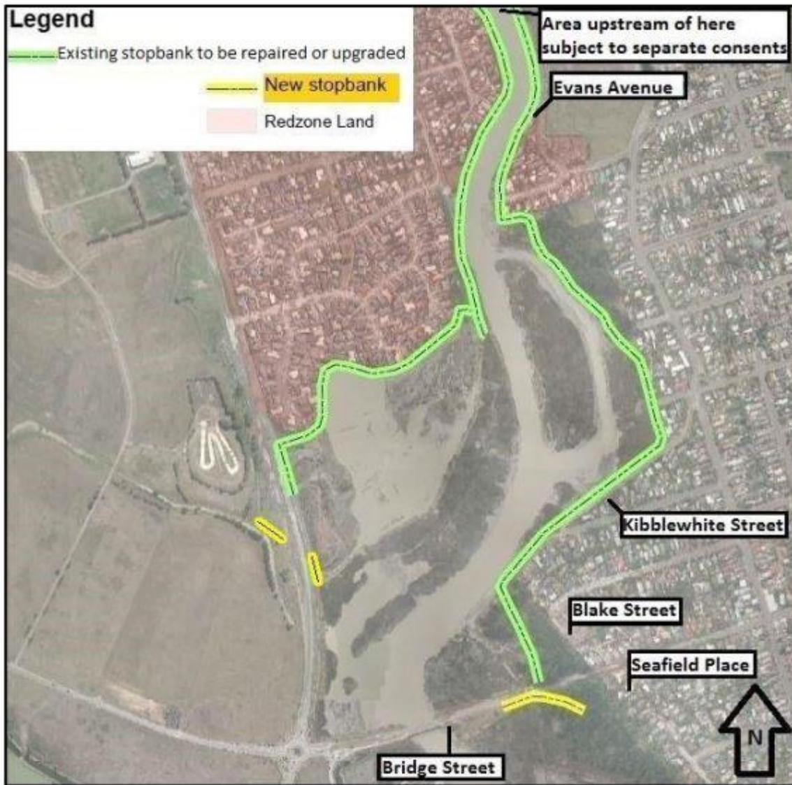
Figure 1 Location of stopbanks to be repaired and upgraded (green) and location of new proposed stopbanks (yellow).
